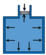
If the top panel is pressed down it applies a pressure to the fluid under it. That pressure presses equally on all sides of the container.
