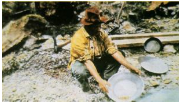
Figure 3. Panning for gold - a process by which a gold minor takes advantage of the process of settling to separate the gold nuggets from the gravel on the stream bed.
